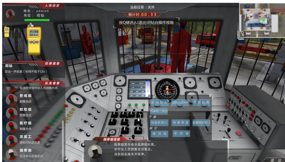
Figure 5 Driller console operation interface
